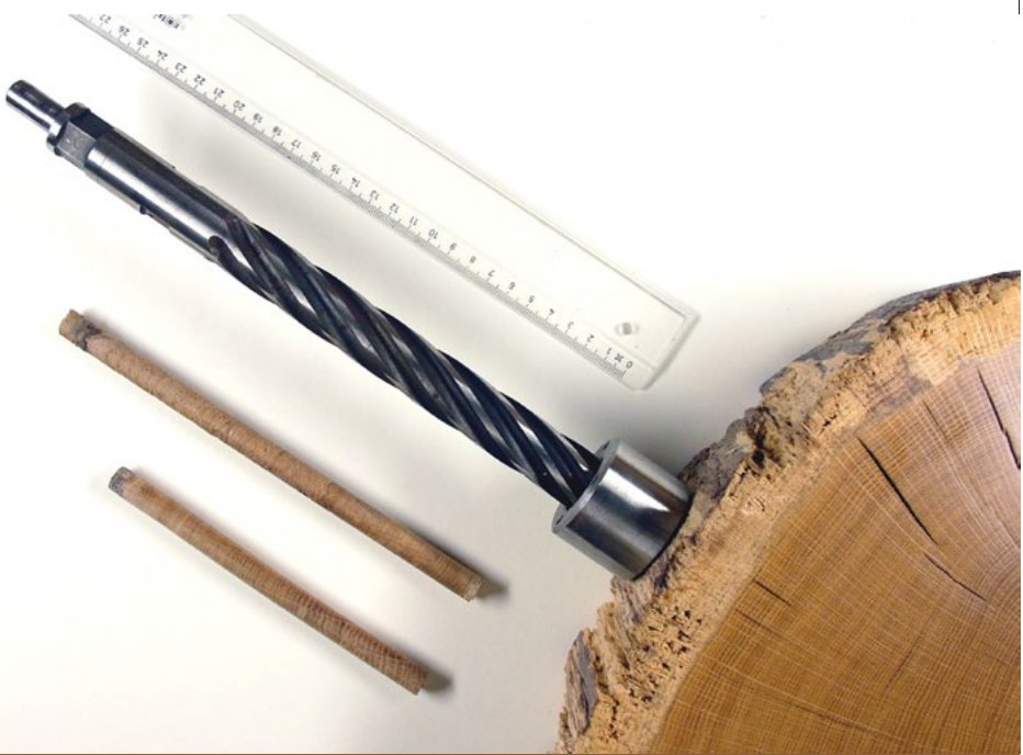
Drill for dendrochronology sampling and growth ring counting Wikimedia Commons
